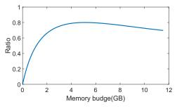
Fig. 6: Ratio of total I/O of MPU and TurboGraph-like.
